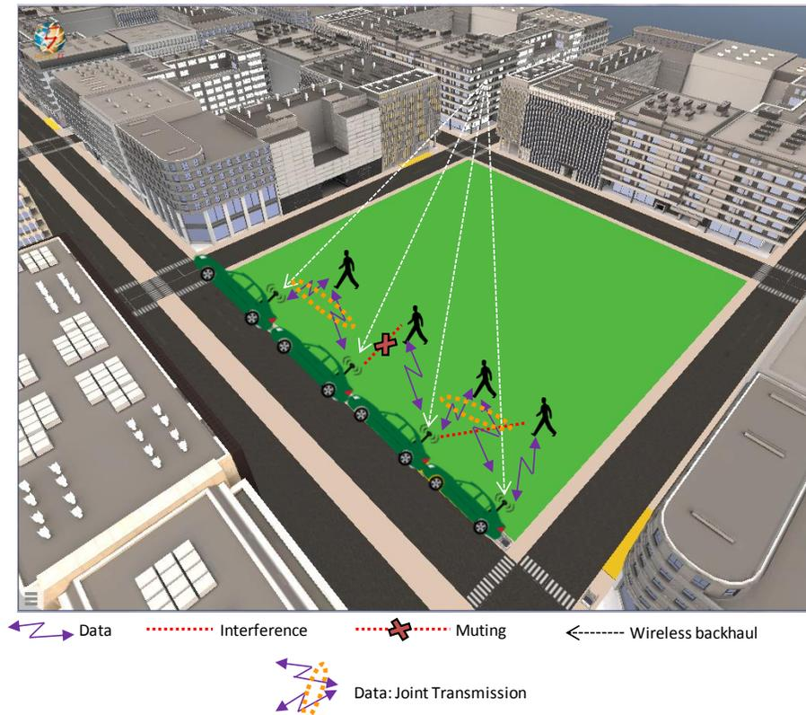
**Figure C-2. Visualization of user-centric interference management in Madrid Grid deployment considering dynamic radio topology based on NNs.**
