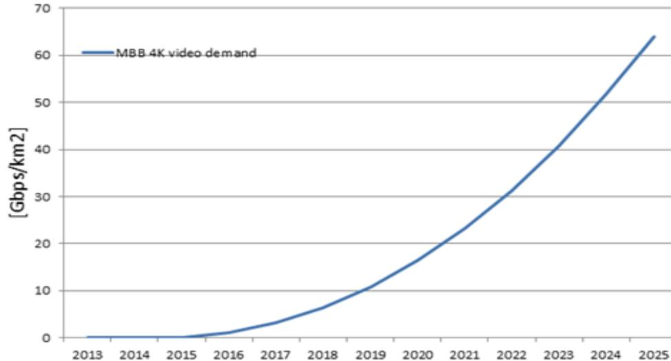
*Example case of xMBB 4K-video traffic up to 70 Gbps/km<sup>2</sup> in the year 2025 shows that bandwidths of at least 500 MHz per operator is needed if the 10 GHz band is used.*
