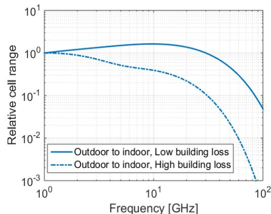
Downlink cell range versus frequency. This indicates that required network densification to cover the area grows with higher frequency.
