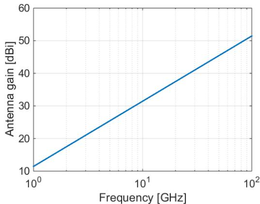
Assumed ideal beamforming gain for a fixed antenna area.
