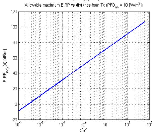
Maximum permitted EIRP as a function of the distance from the transmitter, such that EMF exposure limit given by  $PFD = 10 \text{ W/m}^2$  is not crossed.
