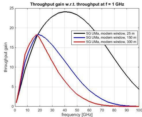
Throughput gain versus frequency. Even with increased channel BW for higher frequencies, throughput decreases after a certain frequency.
