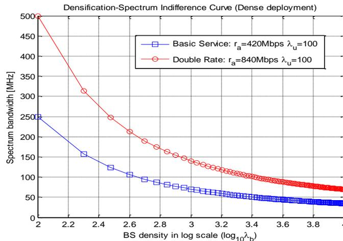
The curves become almost parallel as the BS density increases. This means that it is nearly impossible to increase the user data rate with the densification alone.
