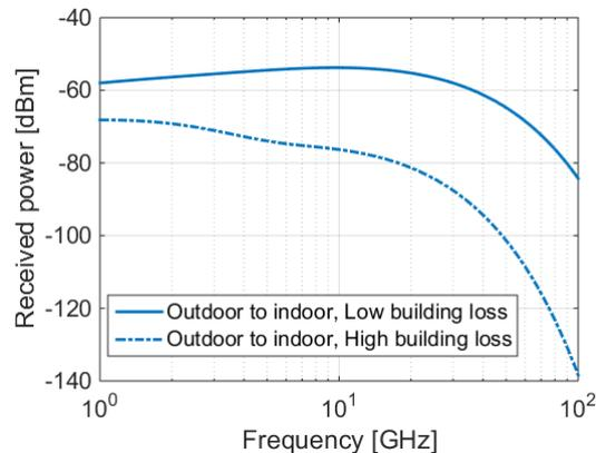
Downlink received power at cell edge versus frequency. Received power decreases even with ideal antenna gain after a certain frequency range.
