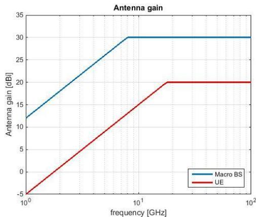
Antenna beamforming gain for a fixed antenna area: Extremely high antenna gains may not be achievable due to challenging management of antenna beams.
