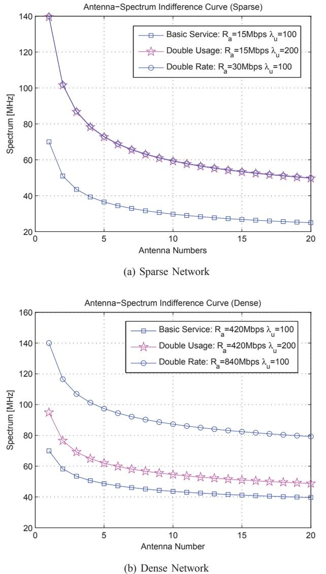
Fig. 2: Relation between spectrum and antenna number.
